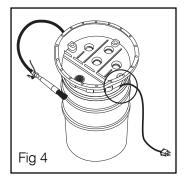
4. Situate the flow-through hose and power cord into the proper slots lined up with wash basin as shown. Make sure that the full length of the power cord is pulled out such that the pump sits flush on the bottom of the bucket, and the full length of the power cord is accessible.
