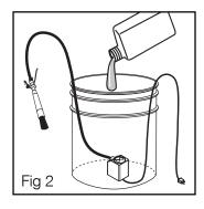
2. Add non-solvent cleaning detergent into the bucket. **WARNING:** Do not use solvent-based cleaners, gasoline, etc.
