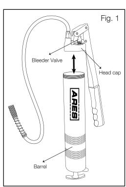
**NOTE:** Apply a generous coating of grease to plunger gasket when using gun for the first time. Due to the lack of lubrication on the rubber plunger, a new grease gun may be difficult to load with grease cartridges the first time. This grease gun requires a 14 oz. grease cartridge.
