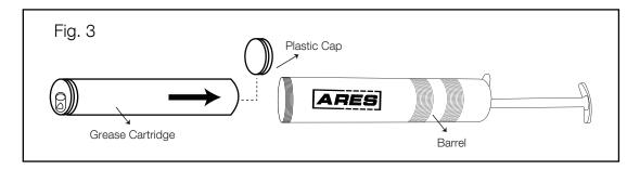
4. Insert the grease cartridge into the barrel completely, making sure the metal pop-top lipped edge tightly seals on top edge of the grease gun barrel. Pull and remove the pop-top seal from cartridge. (Fig. 4)
